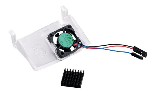
The Raspberry Pi 4 Case Fan is an official accessory for Raspberry Pi 4, for use with the official Raspberry Pi 4 Case. Designed for over-clockers and other power users, it keeps your Raspberry Pi 4 at a comfortable operating temperature even under heavy load.
