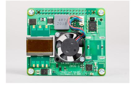
The Raspberry Pi PoE+ HAT is an add-on board for Raspberry Pi computers with PoE pins, including Raspberry Pi 3B+ and Raspberry Pi 4. It is used to power Raspberry Pi via an Ethernet cable, provided that power-sourcing equipment is installed on the Ethernet network. The HAT also includes a fan that will cool the Raspberry Pi processor.
