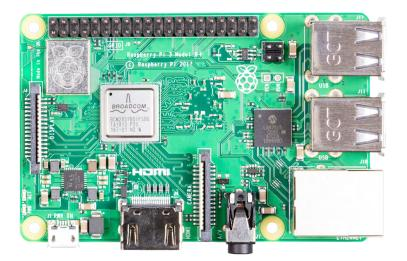
Raspberry Pi 3 Model B+ has a 64-bit quad-core processor running at 1.4GHz, dual-band 2.4GHz and 5GHz wireless LAN, Bluetooth 4.2/BLE, Gigabit Ethernet over USB 2.0, and PoE capability via a separate PoE HAT. The dual-band wireless LAN comes with modular compliance certification.
